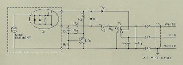
POSITIVE (INWARD) ACOUSTIC PRESSURE PRODUCES POSITIVE VOLTAGE AT PIN 2
