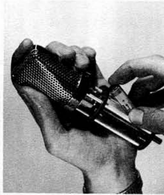
Fig. 8: When replacing batteries, observe polarity markings on the printed circuit board A2. Notice that the two sets of batteries have different diameters and that the construction of the battery bracket makes it impossible to install the batteries in the wrong compartments.
