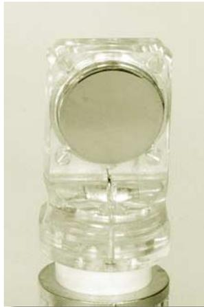
The two existing small diaphragm microphones measure 21 mm in diameter. This dimension served as the basis for developing the next member of this family. The microphone amplifier, or more correctly the impedance converter, does not present a problem. Realizing a switchable microphone however, was a challenge awaiting resolution.
