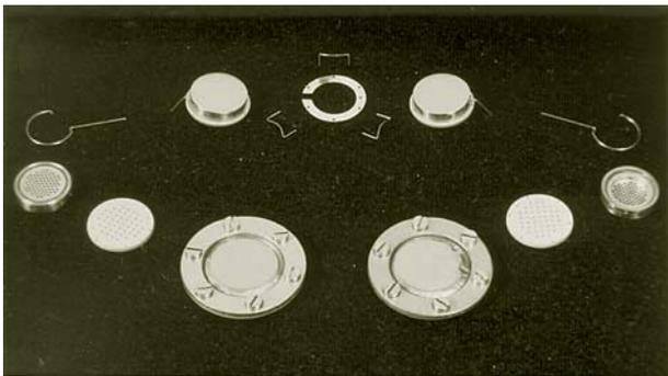
sists of a membrane, back electrode and delay plate. The two capsule halves are mounted together back-to-back with a distance foil, thus forming a dual membrane capsule, similar to the proven M 7 capsule from U 47, U 48 and M 49 fame, but considerably smaller.
