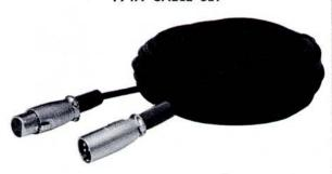
The ALTEC 194A Cable Set consists of a 25-foot length of two-wire shielded, jacketed microphone cable equipped with one XLR3-12 and one XLR3-11C connector. The cable may be used between the base and the power supply, the power supply and the amplifier, or, in multiples as extensions. The 194A can be used with the following ALTEC microphones: M49 through M52 series, 674, 678, 682, 683, 684, 685, 686, 688, and 689 models.
